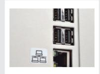
A LAN connection and 4 USB ports for mouse, keyboard, barcode scanner and data transmission
